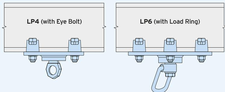
For example, the LP6 has six M24 Type AF clamps to create a Safe Working Load of up to 22,500lbs (4:1 Factor of Safety). Provide details of the loading, rotation, angle and beam dimensions and Lindapter's team of Engineers will design a connection solution to suit your needs.
